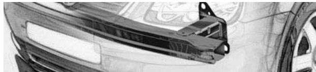
Figure 1. Bumper system consisting of a beam, two crash boxes and a tow nut
