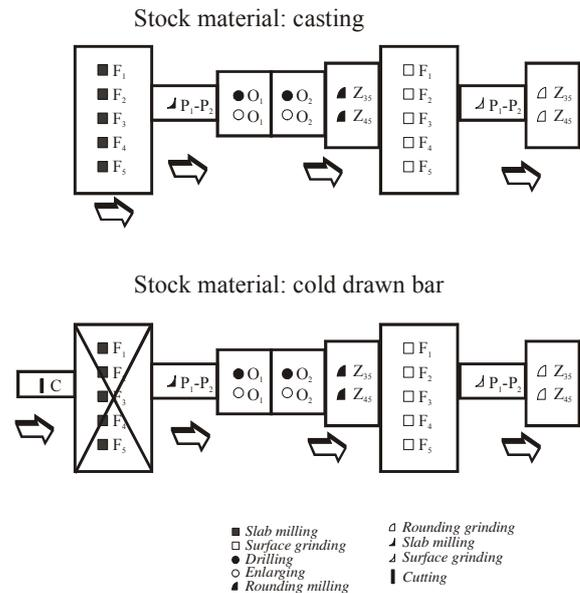
Fig. 3 Example of process part analysis to manufacturing
