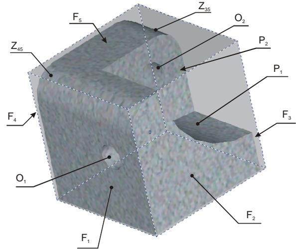
$F_i$  – planes to be machined,  $P_i$  – surfaces,  $O_i$  – holes,  $Z_{ij}$  – fillets
