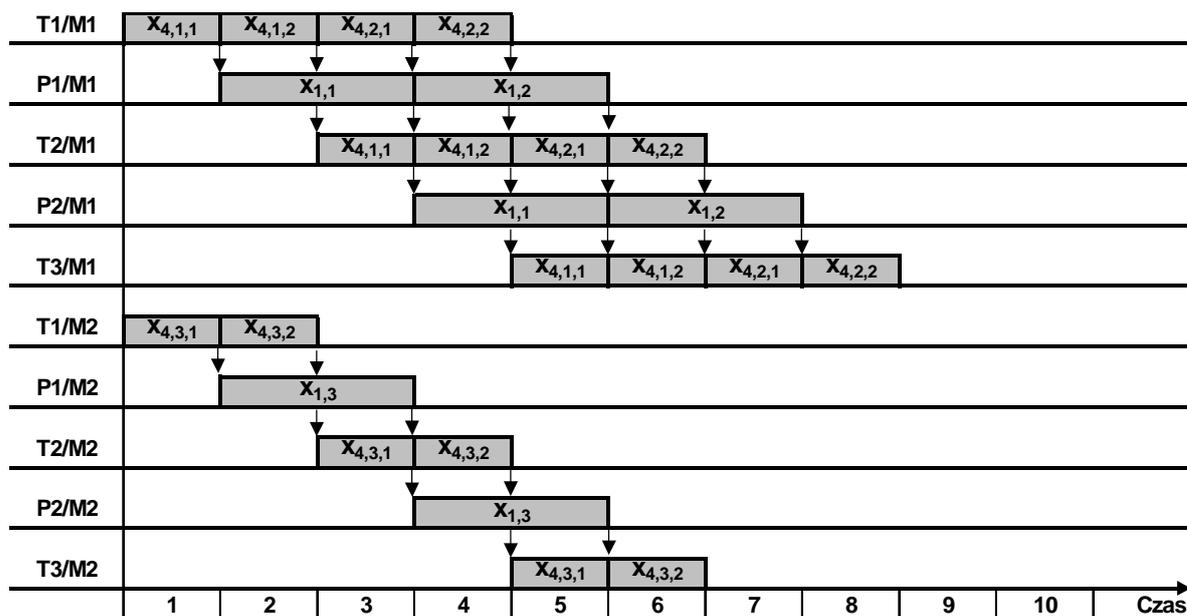
Legend:  $T_i/M_j$  –  $i$ -th transport operation in  $j$ -th routing;  $P_i/M_j$  –  $i$ -th production operation in  $j$ -th routing;  $x_{1,i}$  –  $i$ -th batch production;  $x_{4,i,j}$  –  $j$ -th batch transport of  $i$ -th batch production
