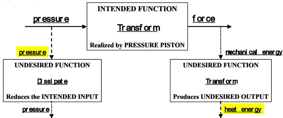
Figure 1. Types of unintended functions originating from principle solutions
