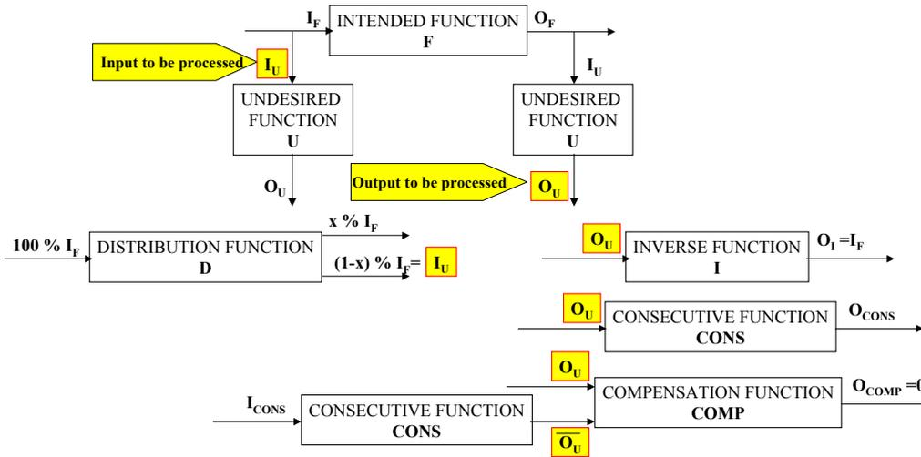
**Figure 2. Processing undesired functions**
