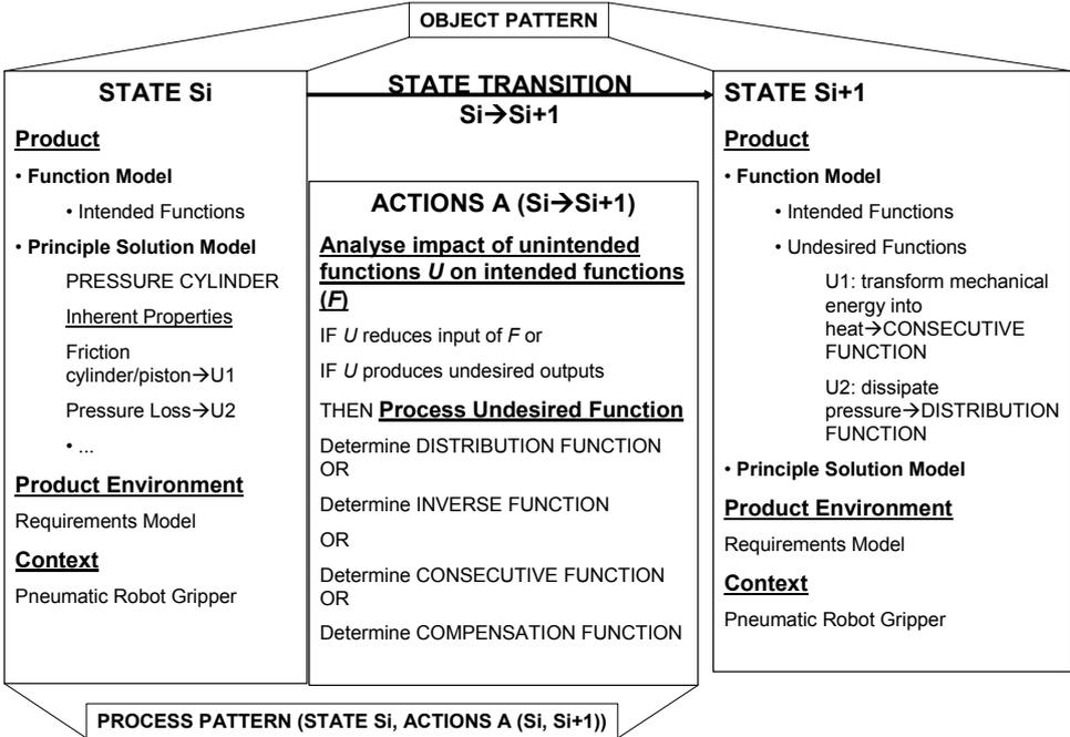
**Figure 3. Relationship between a state transition and object and process patterns**
