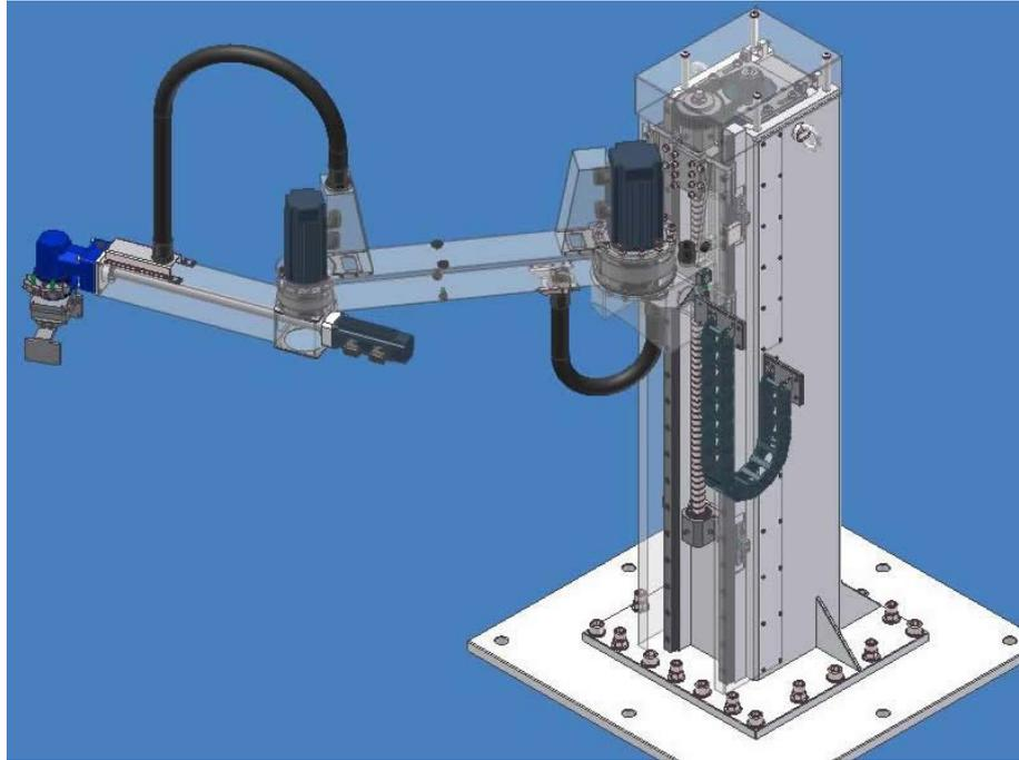
Fig. 4. Virtual prototype of a SCARA robot realised by Engineering students.
