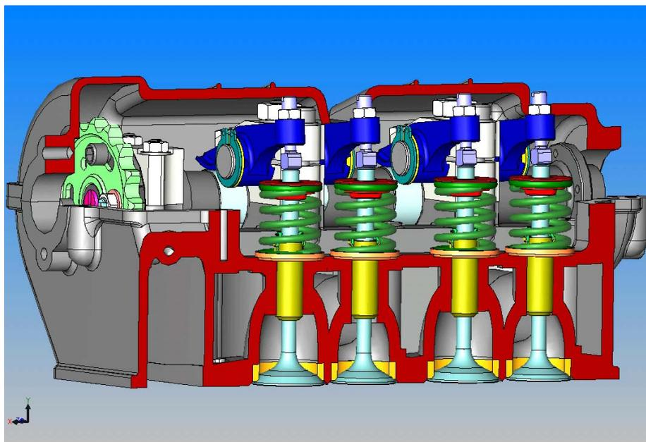
Fig. 5. Valve gear of an engine modelled by 3<sup>rd</sup> year Industrial Engineering students.
