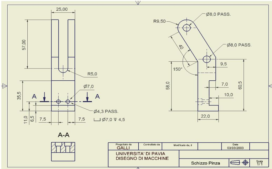
Fig. 2. Drawing of a part of machine shown in fig.1 and used to verify reading ability.
