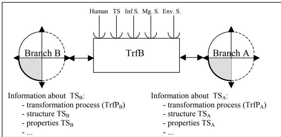
**Figure 11. Principle of the systemic knowledge transfer between two professional TS branches**
