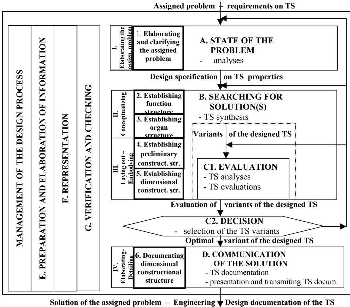
**Figure 7. Basic Structure of the General Procedural Model of the Design Engineering (GMD) of Technical System (TS) (1.-6. Theory of Technical Systems-based Phases) (I. – IV. Traditional Engineering Design Methodical Etaps, A.-G. General Problem Solving Steps)**
