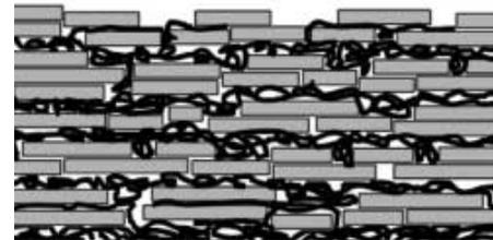
**Figure 3. Illustration of artificial nacre structure [8]**
