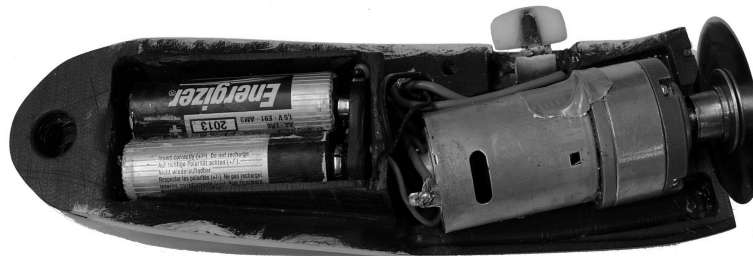
Figure 4 Inside of a powered scissor (prototype)
