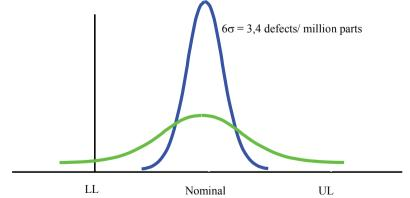
Figure 3 – Process Capability Curve – Conventional versus Six Sigma [8]
