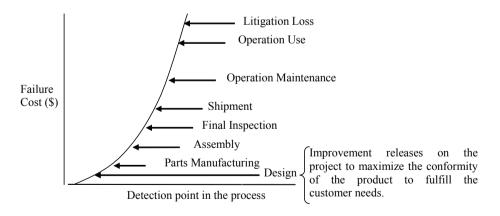
Figure 1 – Failure costs versus failure detection point [2]
