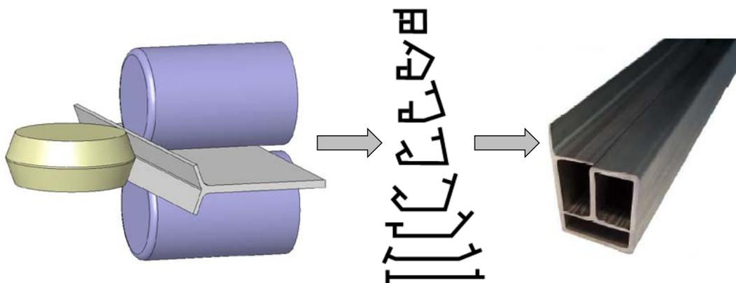
Figure 2: Bifurcated structures with the linear flow-splitting, flower diagram according to [4]
